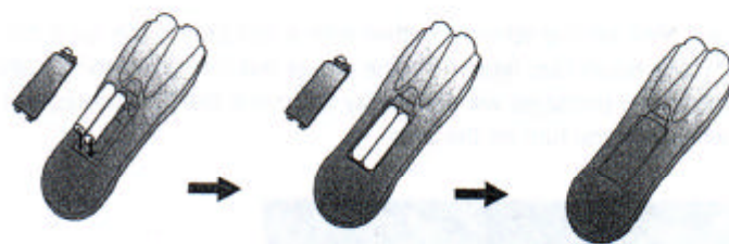
Figure 14 Battery replacement process
